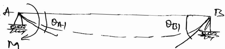
Fig 2. Basic determinate beam Subject to M.
