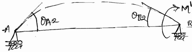
Fig 4 - Basic determinate beam subject to  $M'$
